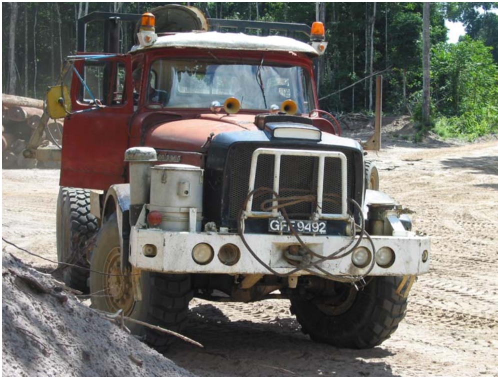
Figure 22: Typical logging truck with rotating amber lights (Note the powerful horns and very visible colours - white top of cab, red bonnet and doors, silver bumper).
